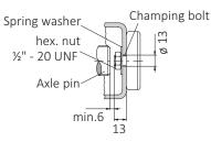
ned clamping bolt is designed for conditions where space is limited.
